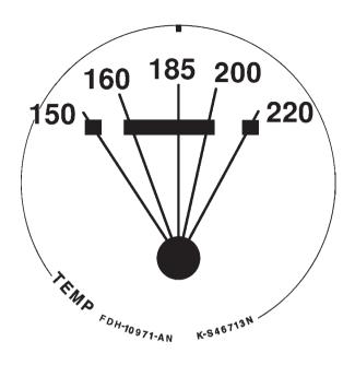
The graphic above shows the approximate temperature in degrees F (+/-5F) that this gauge will indicate for various needle positions. These readings assume that the accessory voltage is 13 volts.
