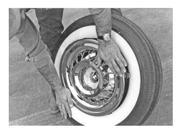
Make sure all clips are locked to the inner flange of the wire wheel and then using both hands, push wire wheel onto the wheel until it snaps into position.
