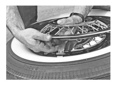
Starting near the top of the wheel, attach clips to wire wheel, pull free end of clip back and away from wheel and hook to inner flange of wire wheel as shown. Attach remaining four clips to wire wheel in same manner.
