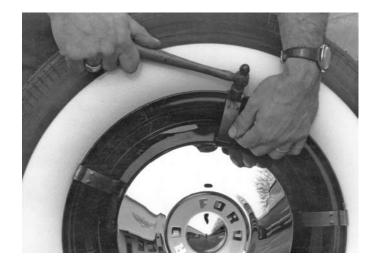
To fasten clips press each clip firmly against the lip of the rim as shown and tap extreme top of clip with a hammer until the clip snaps securely over lip of rim.
