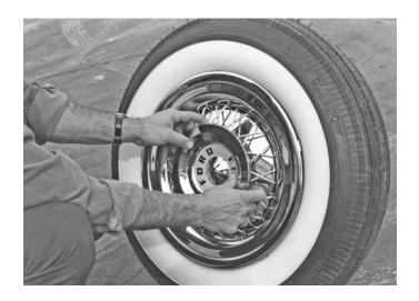
When wire wheel is to be removed or pulled away from the rim, place hands on the collar and spokes and pull out. The spring clips will change phase and hold basket away from wheel assembly.
