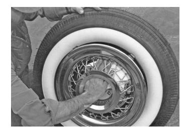
With the wire wheel pulled away from the rim, the air pressure can be checked and the nut cover can be easily cleaned. A clean hub cap will provide the maximum reflection of the wire spokes.
