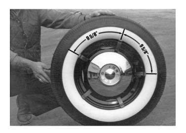
5 clips should be evenly spaced with the valve positioned between two clips. If the balance weights interfere, rearrange spacing positions by placing clips not less than 1/2" from balance weights. Make sure that clip is not installed over top of valve stem.
