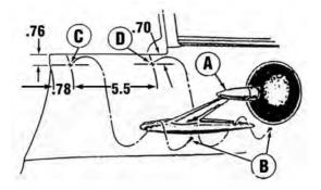
A - 17696 mirror assembly - rear view outside one required left side of car only.
