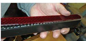
6. Apply a small amount of silicone sealant to the cover pocket on the bottom of the housing. Install the pocket cover, making sure that the wires have a bit of sealant on them where they exit the housing. Using a couple small pieces of masking tape, lightly tape the cover on while the sealant cures.
