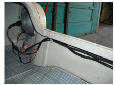
3. At the LH lamp, remove one of the nuts from the lamp housing and secure the grounding eyelet. LED's require very good ground connections. Make sure that this connection is a good ground.
