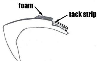
Position the foam on the header as shown – note the taper is toward the rear.
