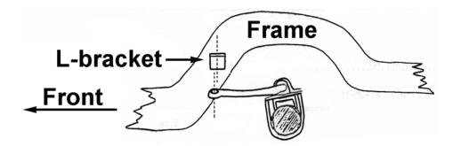
With hole aligned, weld or drill and bolt "L-bracket" to frame. Then install bolts and bushings. Next tighten "U-bolts" on axle housing. Replace rear wheels and remove jack. Check to make sure that all bolts are tight.
