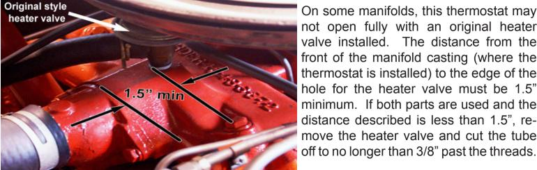
On some manifolds, this thermostat may not open fully with an original heater valve installed. The distance from the front of the manifold casting (where the thermostat is installed) to the edge of the hole for the heater valve must be 1.5" minimum. If both parts are used and the distance described is less than 1.5". remove the heater valve and cut the tube
