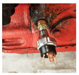
Remove the hex socket head plug in the oil rail located nearest the fuel pump as shown. In the example pictured some heat was required to persuade the plug to let go.
