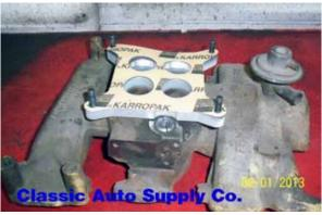
Place the smaller carburetor to intake manifold gasket on intake manifold. Insert allen head screws in adapter plate and install adapter plate to intake manifold making sure notch on adapter plate is on the side where automatic choke assembly was previously removed. Place the larger carburetor to intake manifold gasket on adapter plate.
