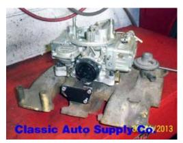
Install new vacuum line from intake manifold fitting to fuel pump. Install new carburetor.
