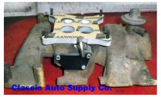
Install choke heat tube adapter into well where 9820A choke tube was previously removed. Install choke blockoff plate. Make sure air pin hole in plate is open.
