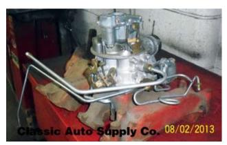
Remove carburetor, 9820B choke tube, fuel line from carburetor to fuel filter, 9877 choke tube elbow, 9820B choke tube and all vacuum lines.
