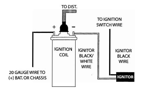
WIRING DIAGRAM FOR SYSTEMS WITHOUT BALLAST RESISTORS
