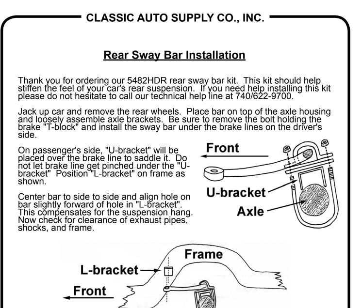
With hole aligned, weld or drill and bolt "L-bracket" to frame. Then install bolts and bushings. Next tighten "U-bolts" on axle housing. Replace rear wheels and remove jack. Check to make sure that all bolts are tight.
