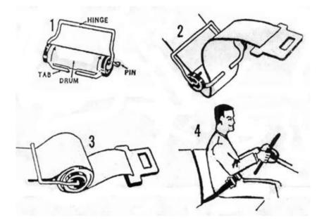
**Warning** - Seat belts must be worn tight! After installing, make sure that no webbing remains on the retractor when belt is in use.
