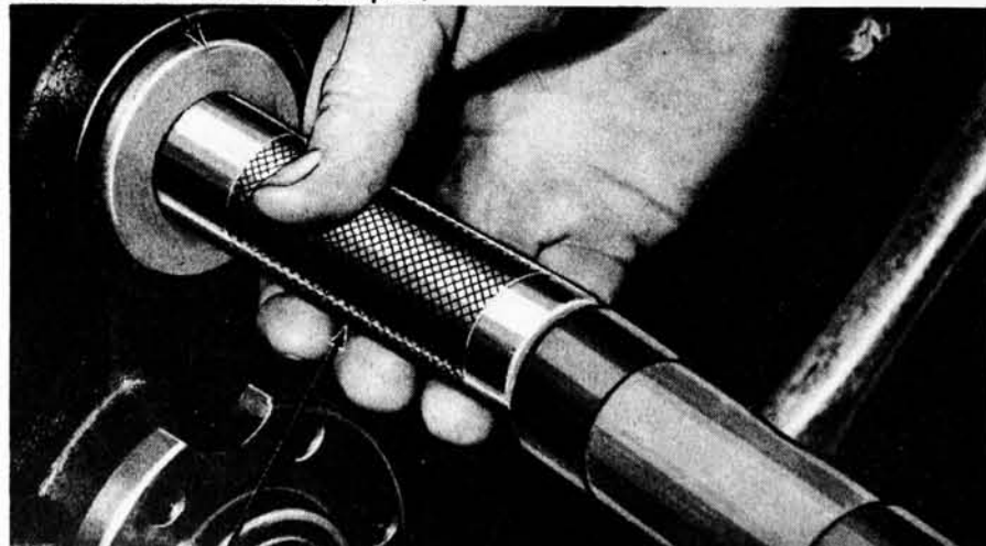
Fig. 22—Camshaft Rear Bearing Bore Plug Removal
