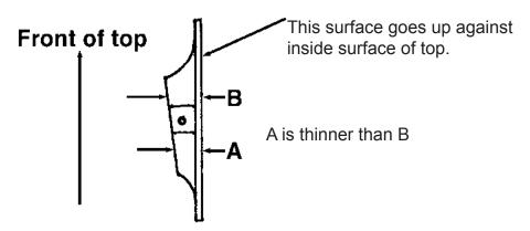
B. Attaching. Secure porthole spacer with resin. It is recommended that the surfaces to be mated be ground or sanded with course paper to roughen the surface. Glass cloth or mat may be added to strengthen if desired.
